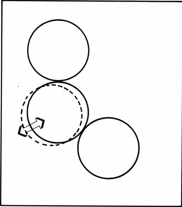
Moreover, by means of a second excentric bearing it can be moved towards the impression cylinder.
