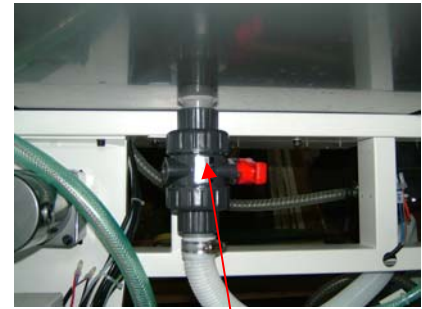
Chemical drainage valve
