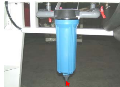
Lowest chemical drainage valve
