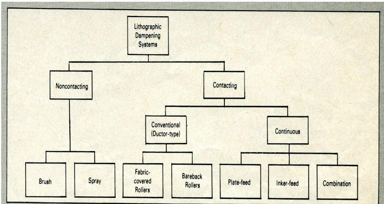
*Figure 1: Classifies litho dampeners under the general headings of non-contacting and contacting systems, and the latter into conventional and continuous types.*
