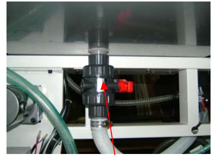
Chemical drainage valve
