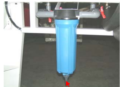
Lowest chemical drainage valve
