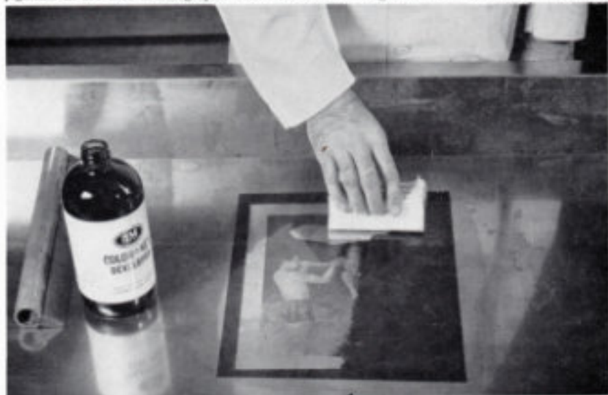
After removing the coating in the non-image areas the sheets of Colour Key are rinsed with water and dried with a soft cloth. The same developing process is followed with each of ten colours available
