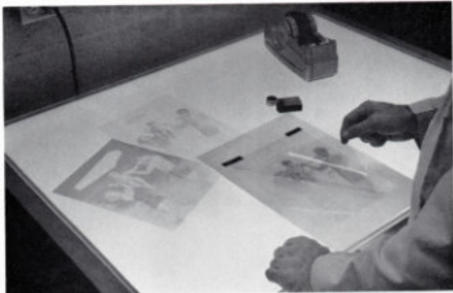
Colour Key sheets are placed down in the same order that the inks will be run, and employ the same pigments as are used in lithographic inks. Each sheet has registration marks for exact alignment
