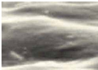
Glazed roller with calcification on the surface
