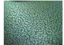
Cracking due to chemicals
