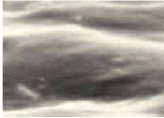
Glazed roller with calcification on the surface
