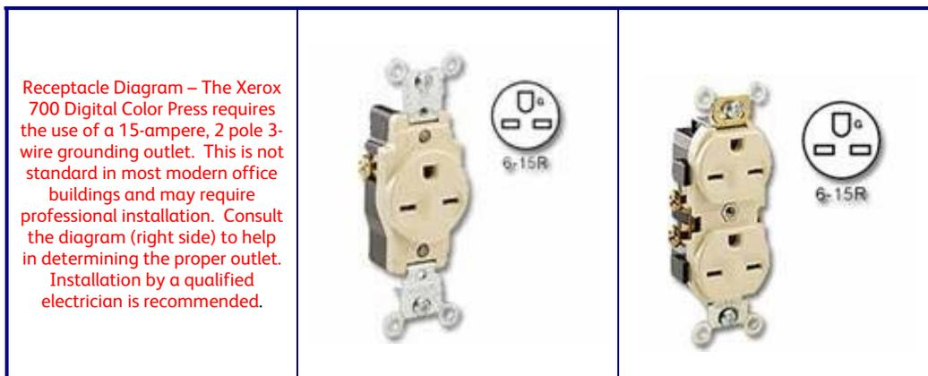
A single power cord (see above) is required for the Xerox 700 Digital Color Press. With the exception of the HCF, Advanced Finisher and Professional Finisher, each optional feeding and finishing device requires an additional 100-240VAC minimum 240VA circuit with a Nema 5-15R receptacle (standard in US) or flying-leads.
