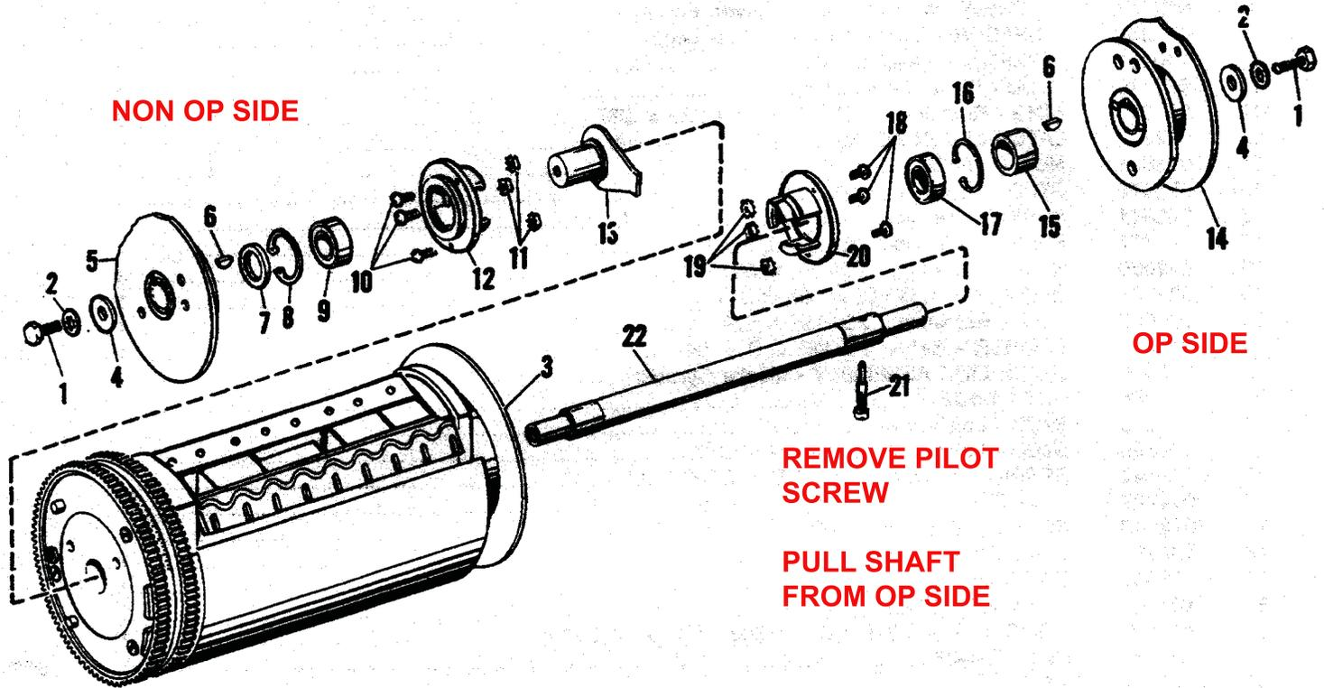
I use a special tool to remove the shaft, It is basically a piece of pipe that goes against the side of the cylinder and has a threaded part that screws into the end of the shaft thru the pipe and a large washer and nut that applies pulling pressure against the side of the cylinder.
