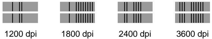
Figure 3.3 Bar codes indicate the resolution (dpi value) used to image a test page.
