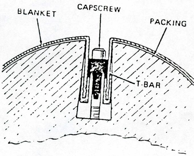
Figure 13. T-bar lockup system
