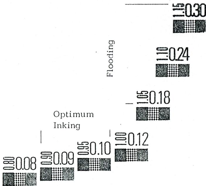
It is extremely difficult to determine optimum inking optically, especially as regards yellow. The Brunner measuring strip safely detects the beginning of flooding because of the fast increase in dot enlargement (concrete example for yellow).
