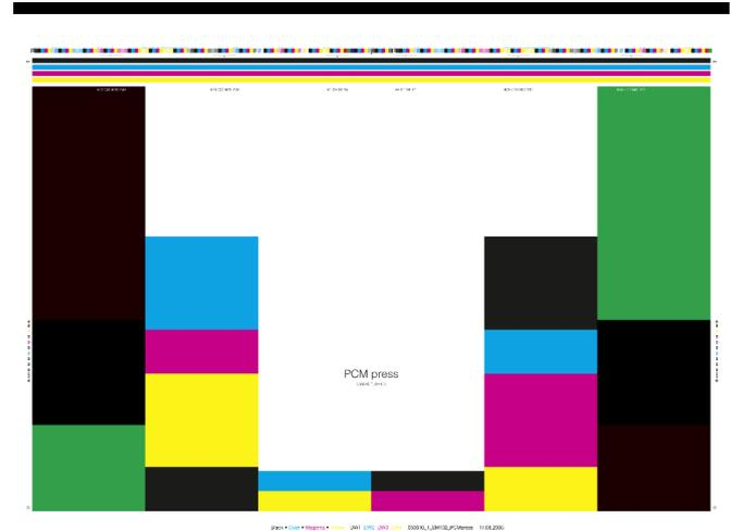
Print the sheet as the ppf file with no adjustment to the ink keys, but with the press at a stable condition and speed.
