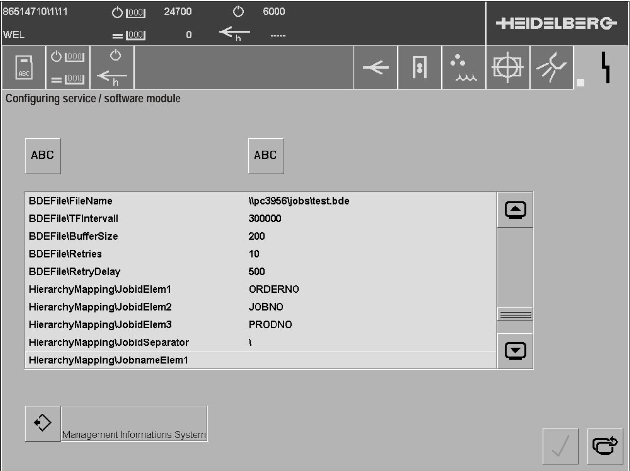
Fig. 8 "Configuring software modules" service display with connection to MIS, part 2
