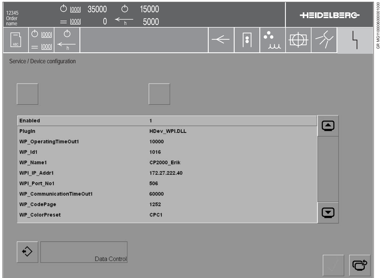
Fig. 6 "Configuring device" service display with connection to DataControl
