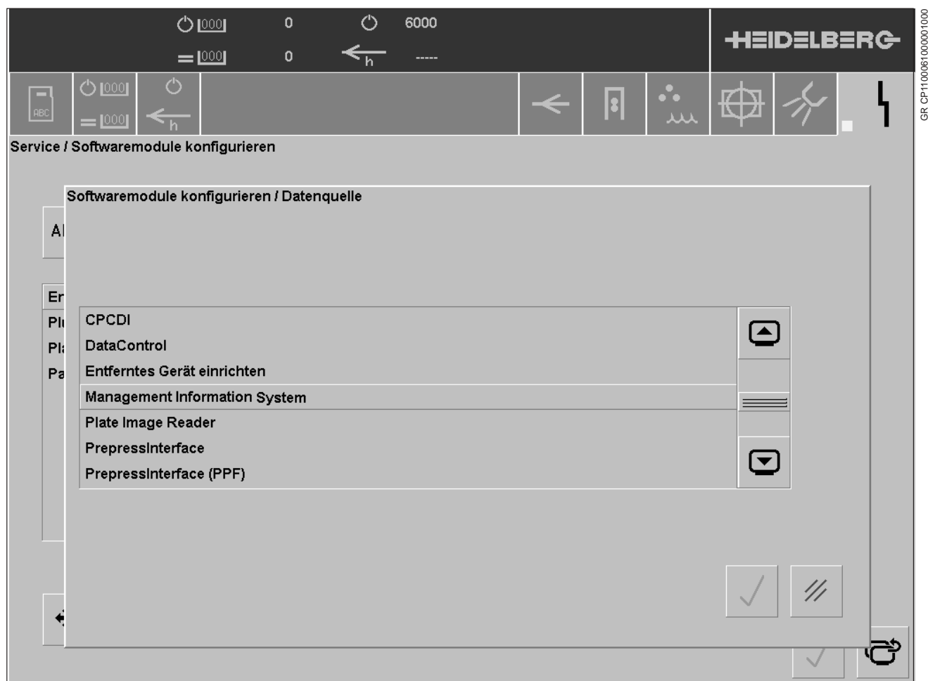
Fig. 5 "Configuring software modules / Data source" service display
