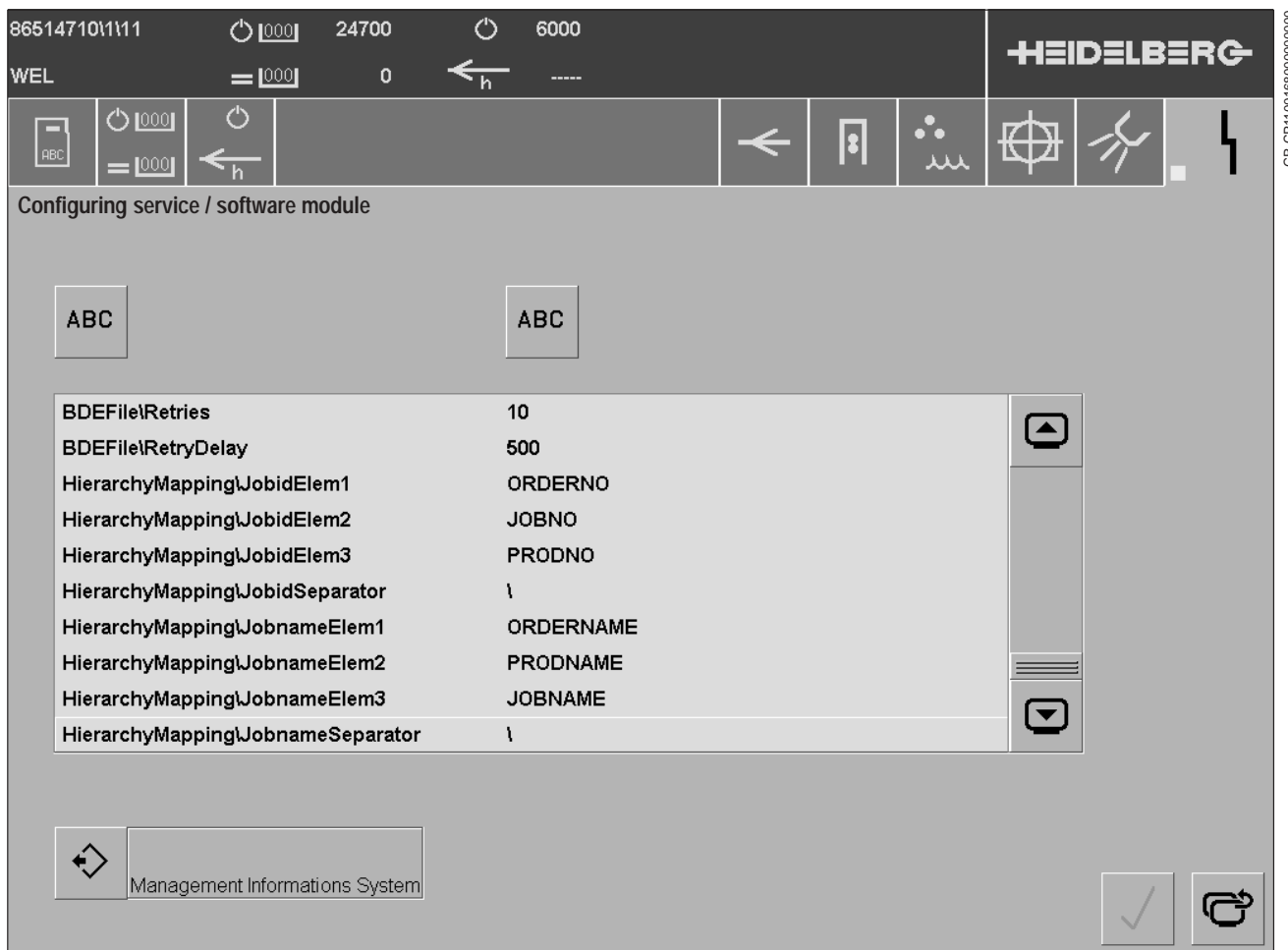
Fig. 9 "Configuring software modules" service display with connection to MIS, part 3
