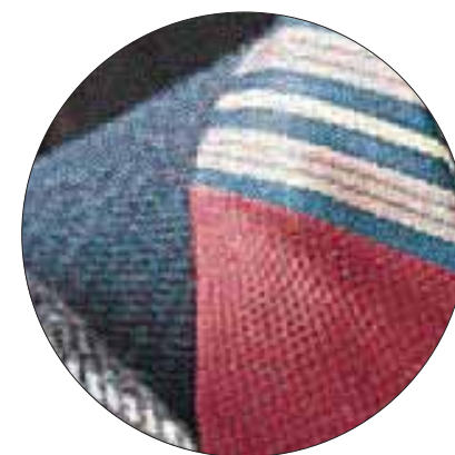
Figure 55: Enlarged section from the FM screen (Prinect Stochastic II fine).
