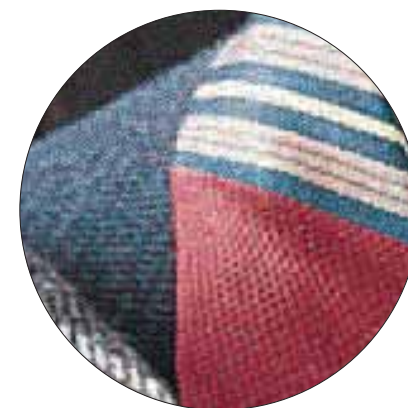
Figure 58: Enlarged section from the Prinect Stochastic Screening II fine screen.
