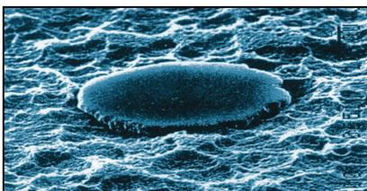
screen dot on non-printing aluminium oxide
