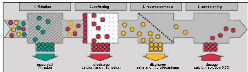
Fig. 5: Principle of process water treatment using the example of reverse osmosis
