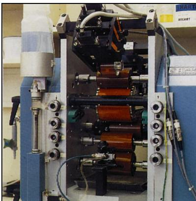
Fig. 20: LithoLab tester for investigation of ink/water balance
