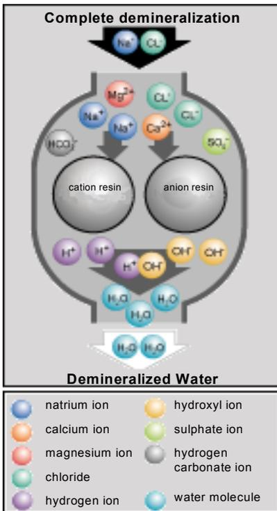
Fig. 4: Principle of complete demineralization
