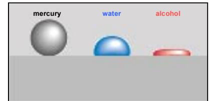
**Fig. 13: The surface tension of liquids determines their wetting behaviour**
