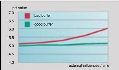
**Fig. 9: Stabilization of pH value by good buffer capacity**
