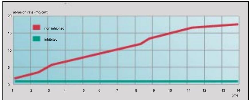
Fig. 19b: Determination of nickel mass loss. Practical behaviour of inhibited and non-inhibited systems
