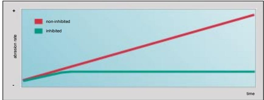
Fig. 19a: Determination of nickel mass loss. Theoretic behaviour of inhibited and non-inhibited systems
