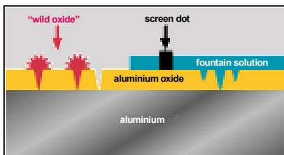
**Fig. 12: Formation of plate corrosion**
