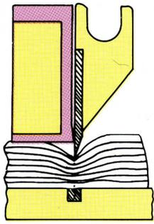
*As a consequence of too low pressure or insufficient initial clamping, the knife, when engaging, compresses the material further before it is cut.*
