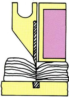
As a consequence of too low pressure on soft stock and depending on the sharpness of the knife and the pliability of the material, a difference between the top and bottom layers will occur, usually an undercut or a pull.
