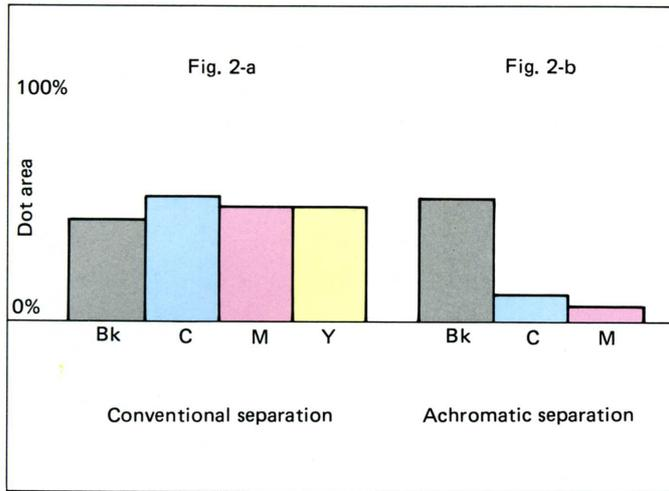
If the reproduction of the Black colour, by 100% Black ink only, lacks saturation or gloss, we can overcome this by either using a stronger pigmented black ink or we can reintroduce any desired value of Yellow, Magenta and Cyan to reinforce the Black. This colour Black addition is confined to the neutral tones only, and has no effect on the colours.
