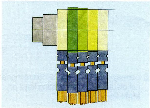
They are arranged side to side with minimum gap. Their front edge is made of wear-resistant material. Each slide is individually adjustable, forward and backward. The adjusting operations do not influence the position of neighbouring slides.
