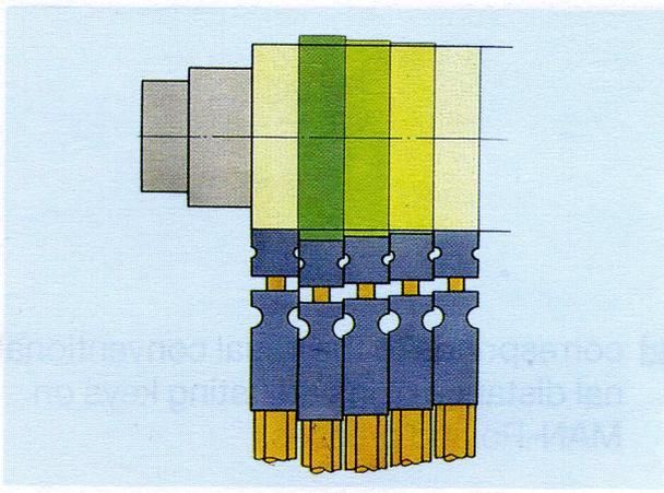
They are arranged side to side with minimum gap. Their front edge is made of wear-resistant material. Each slide is individually adjustable, forward and backward. The adjusting operations do not influence the position of neighbouring slides.
