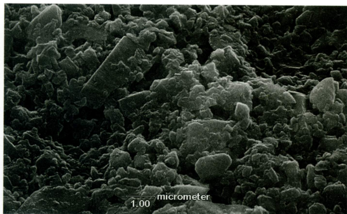
Fig. A6 10,000-fold magnification of the paper surface of Magno Satin .
