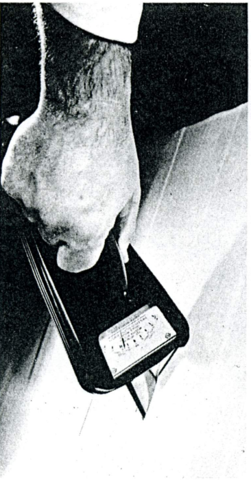
Figure 37: The GATF Paper Hygroscope being used to test the moisture balance of paper.
