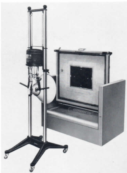
Above right, a Lithotex whirler, used for coating plate surfaces with light sensitive solution; above left, a printing down frame with glass in raised position; and below, a plate being exposed
