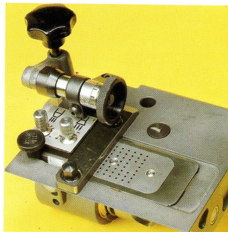
The patented pneumatic sidelay.
