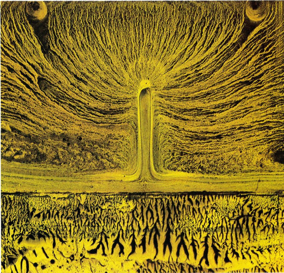
*The pattern shown in this gap current largely corresponds to the flow pattern close to the zone near the the pneumatic sidelay. The blow/suction nozzle thus serves here to stabilize the sheet edge. The view is - so to speak - through the sheet to this nozzle which is faintly visible in the picture centre (round outline).*
