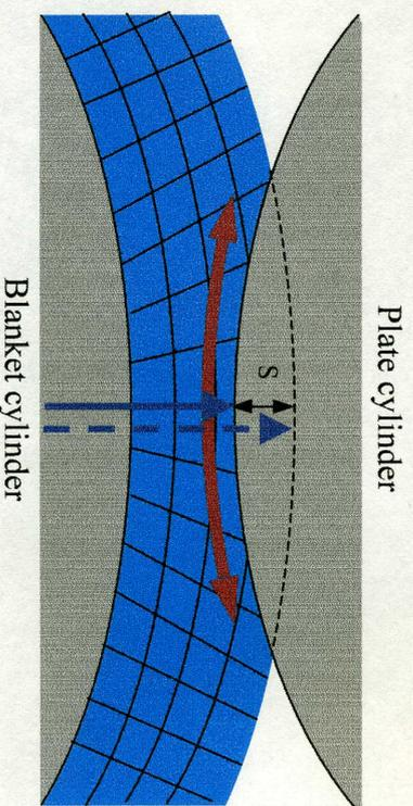
Stretching of the incompressible rubber medium (eff. Diameter )
