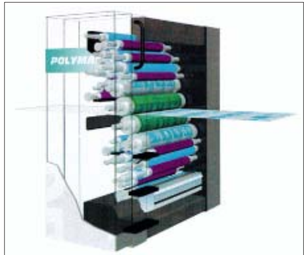
Double sided printing in a printing unit
