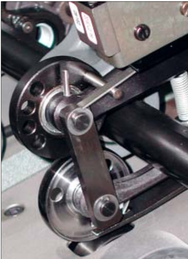
Double sheet detector
