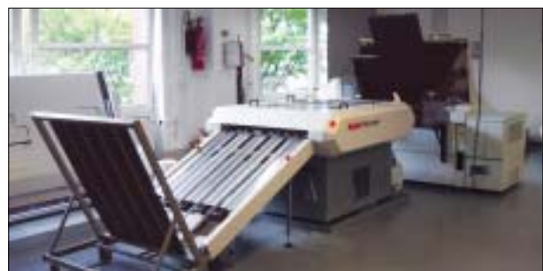
On this equipment, the image is transferred to the printing plate
