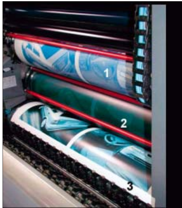
Printing unit with printed sheet on the impression cylinder: 1 Plate cylinder 2 Blanket cylinder 3 Impression cylinder with a printed sheet
