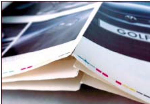
Breaking at the fold
