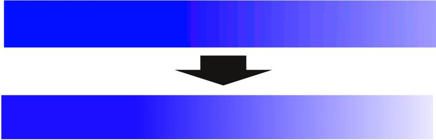
Gradations can sometimes print a bit blocky or not as smooth as they appear on your screen. This can sometimes be down to the source file not being created particularly well or the RIP not processing the image efficiently.
