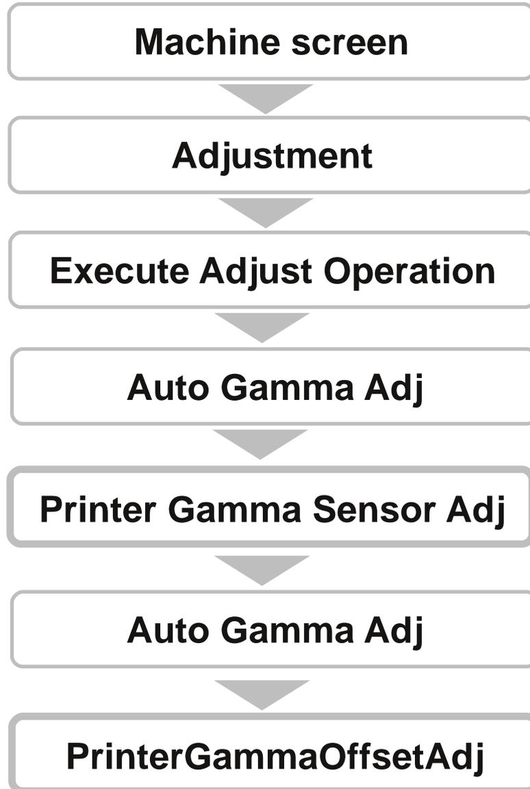
Printer Gamma Sensor Adj and PrinterGammaOffsetAdj are explained in this handbook. The second Auto Gamma Adj is just a repeat of the first Auto Gamma Adj.
