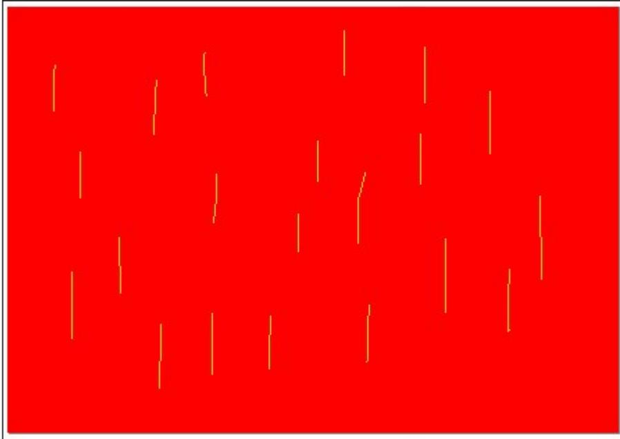
When printing at maximum density for example 100% Magenta and 100% Yellow you might see some random deletions or lines on the print. This is usually worse in an extremely dry environment. Adjust the front back density to counter this.
