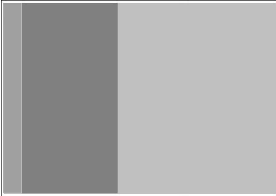
This mainly happens on heavy stocks. An unusual dark banding an about a inch wide from the lead edge and another halfway across the page. This seems to be humidity related. To cure this adjust the separation DC front back setting to a negative value.
