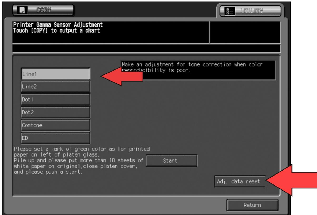
Step 2. Select line 1, select copy, print out the test chart on letter/a4 and place the test chart on the scanner glass with the green arrow to the left, place 10 sheets of paper behind the print and close the glass.
