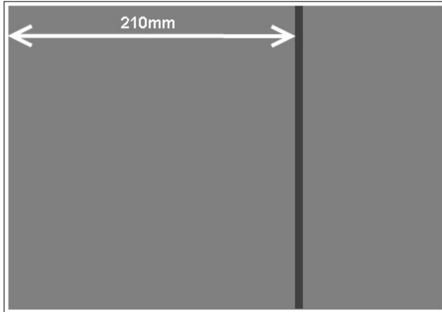
To prevent a black band from appearing when printing on thick stocks in b&w mode turn on thick black mode.
