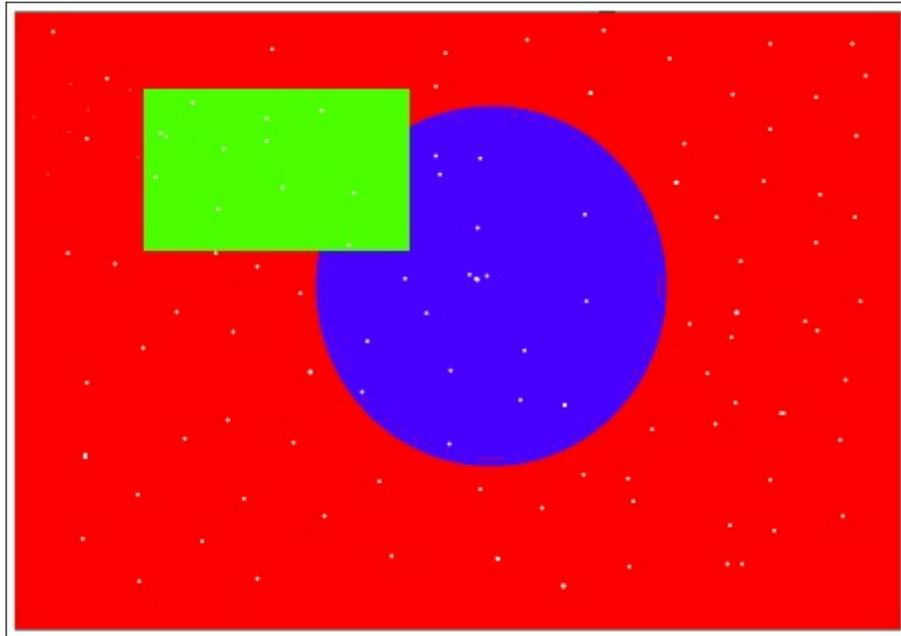
On some stocks white dots might appear in solid areas, this may only effect one side of the print. To avoid this adjust the 2nd transfer offset adjustment for each side until the effect disappears.
