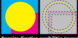
Trapping direction possibilities (spread out, choke in) are shown as dashed lines. Trapping is calculated depending on what ink types are used on touching objects...
